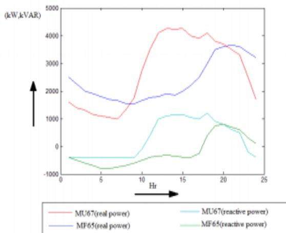
Fig 5. Power profiles of Feeder MF65 and MU67 (w/o FC system).
