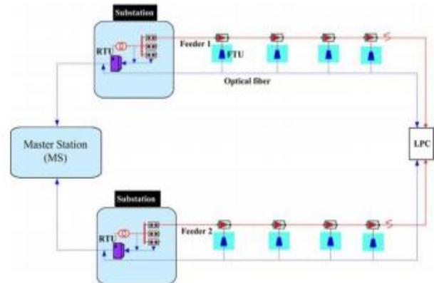
Fig 3. Distribution automation system with a loop power controller
