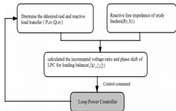
Fig 4. Flowchart of LPC control algorithm
