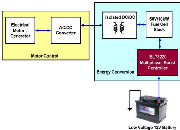
Fig 2. Detailed block diagram of the fuel cell system
