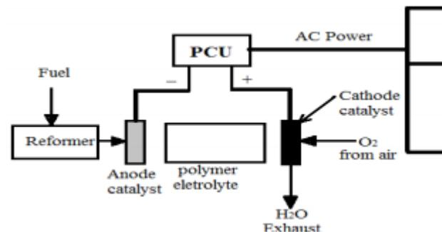
Fig 1. Configuration of the fuel cell system
