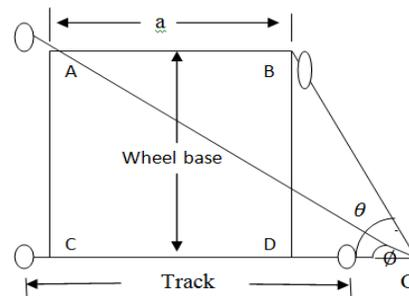
**Fig: 1.1. Condition for true rolling:**
