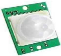
**Figure 3. Motion Sensor**
