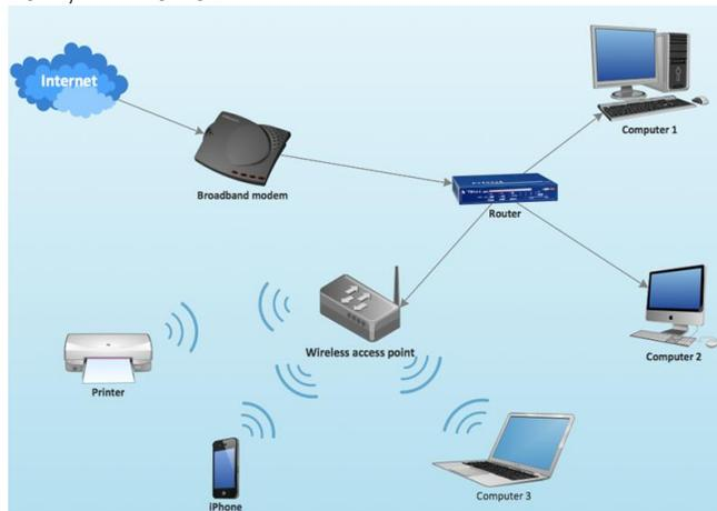
Fig 1. Hybrid Home network diagram
