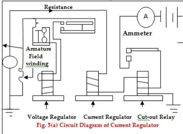
Fig. 5(a) Circuit Diagram of Current Regulator
