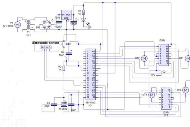
Fig 2. System architecture of Mobile Robostick
