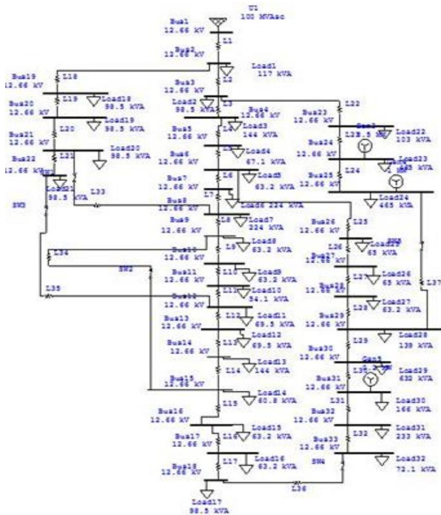
Figure 6. 33 Bus Systems with Tie Lines and DG
