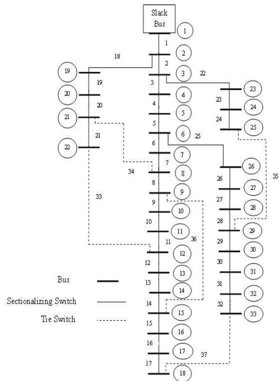
**Figure 4. 33 Bus Radial Distribution System**
