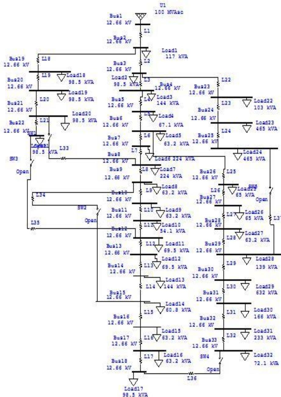
Figure 5. 33 Bus System Base Case
