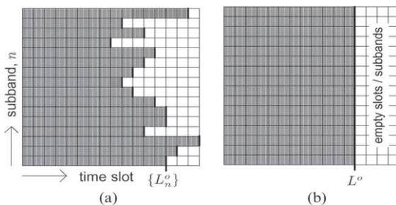
Fig.2 . Illustration of the proposed EMA. a) Fine-EMA algorithm: SDMA with  $1 \leq L_n^0 \leq T$  or TDMA for each subband b) Coarse-EMA algorithm: SDMA with  $1 \leq L_n^0 \leq T$  or TDMA
