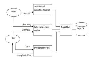
Figure 1. System Architecture
