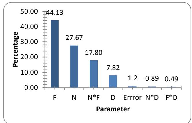
Figure 6: Contribution of parameters on surface roughness
