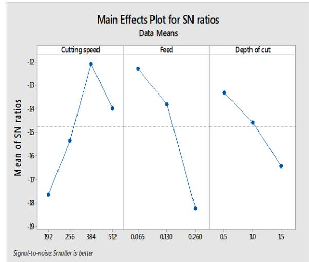
Figure 5: Main effect plot for SN ratios
