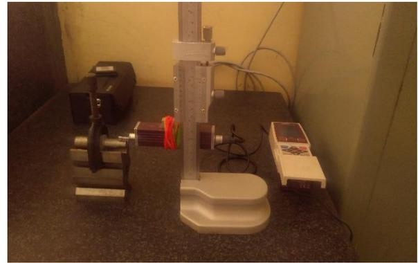
Figure 2: Surface roughness measurement
