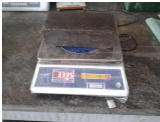
Figure 6. Weight of dry brick
