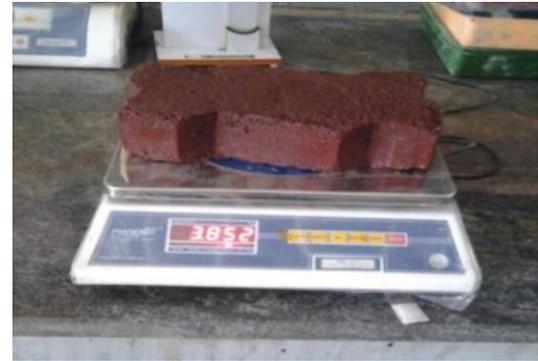
Figure 7. Weight of wet brick
