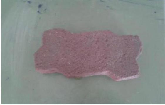
Figure 8. Efflorescence test for plastic-sand brick
