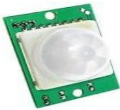
**Figure 3. Motion Sensor**
