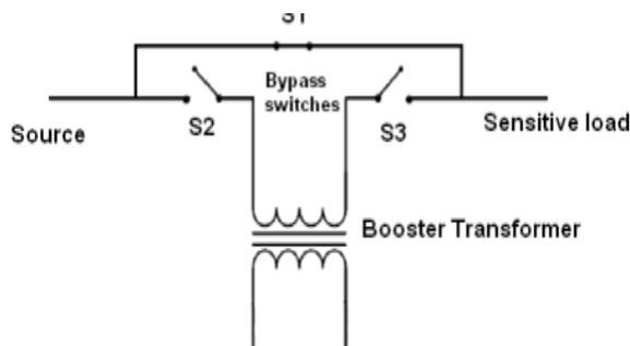
Fig. 5 Protection Mode (creating another path for the load current)
