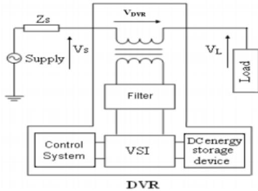
Fig. 4 Dynamic Voltage Restorer (DVR) general configuration
