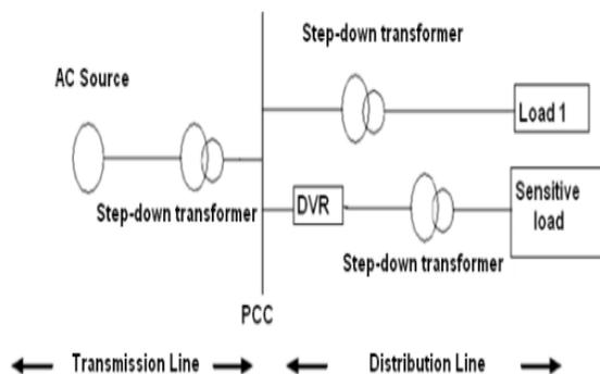
Figure 3 .location of dynamic voltage restorer (DVR) in an electrical power system.
