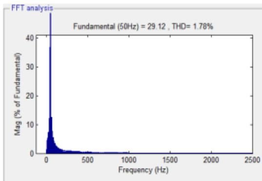
Fig 5.8: FFT analysis of grid current with out fuzzy
