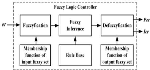
Fig 2. Block diagram of basic FLC.
