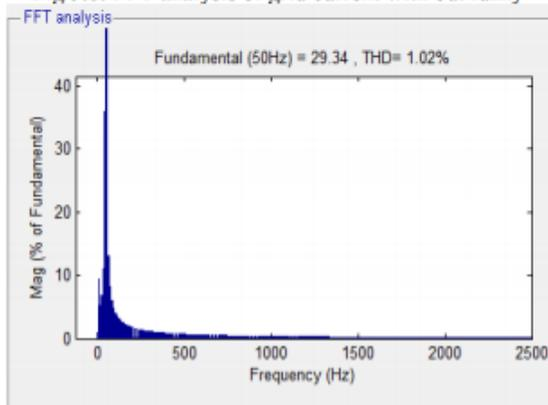
Fig 5.9: FFT analysis of current voltage with fuzzy The THD of without fuzzy is 1.78 and with fuzzy is 1.02
