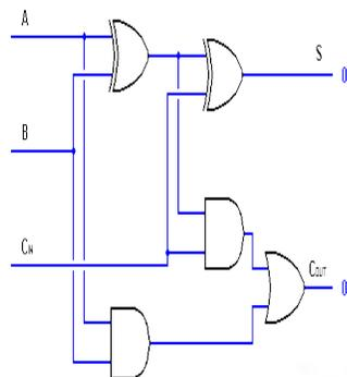
Fig.4. The gate level implementation for explanation of full adder
