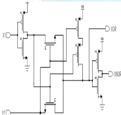
Fig.2. Circuit diagram of XOR-XNOR
