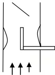
This type of carburetor is fitted under the manifold and it is mostly fitted for Industrial engines.
