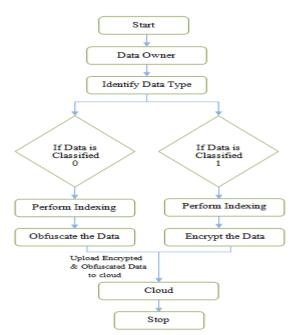
Figure 3.2 Encipher and Indexing
