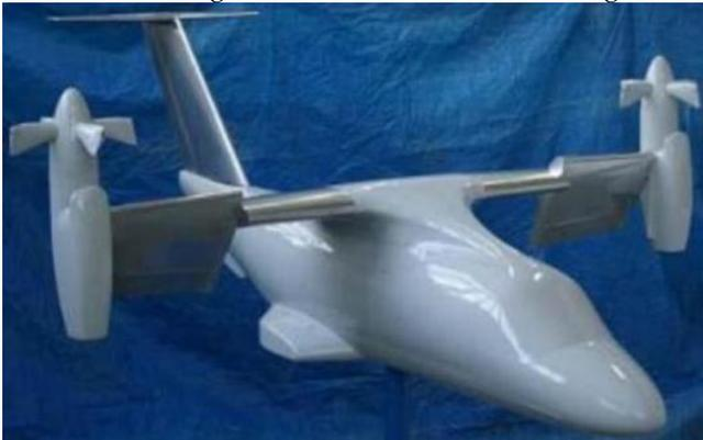
Figure 1: Complete model of an aircraft made by R.P [3]
