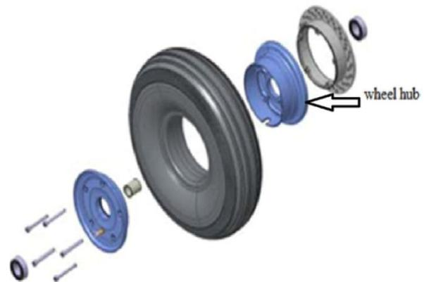
Fig 2.1 : Position of Wheel Hub
