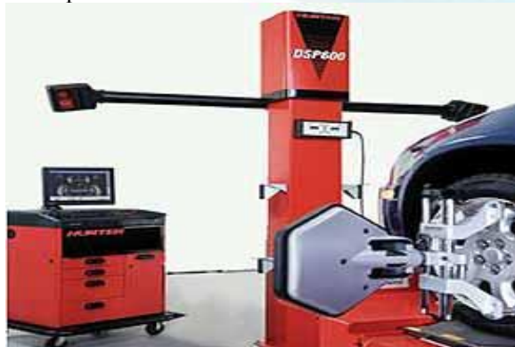
Fig. 5(a) Wheel alignment procedure. ( Source: www.platinumautoservice.com )
