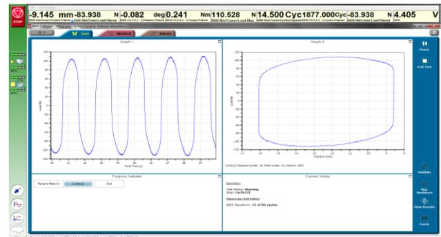
Fig no.6 Damping force-deflection curve at 1A
