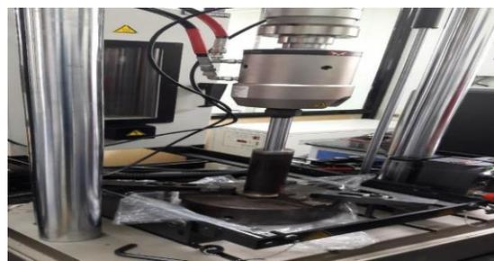
Fig no. 3 The Fatigue testing machine
