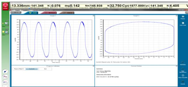
Fig .no 5 Damping force-deflection curve at 0.5A
