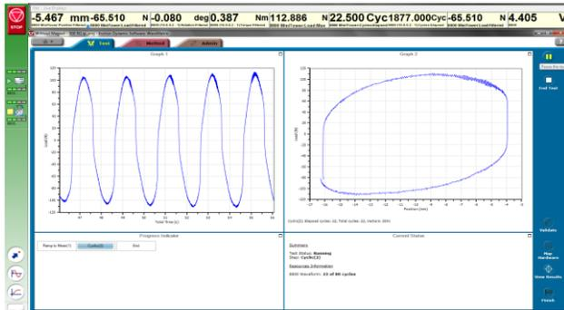
Fig no.4 Damping force-displacement curve at 0A
